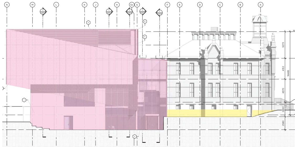
Proposed west elevation, showing new construction in pink, change in grade and foundation to be exposed in yellow (RAW, 2019; Annotated by ERA, 2019).
