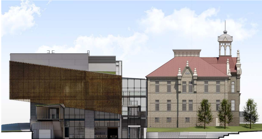
Figure 2 - West Elevation with Aged Muntz Bronze
