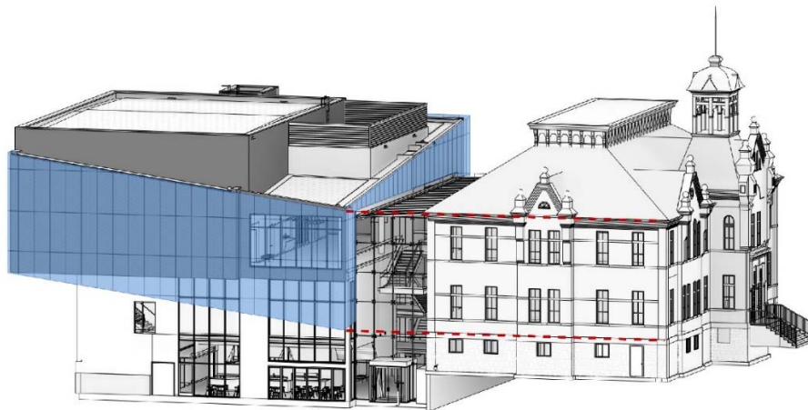
Figure 8 - Application of the Veil over the façade
