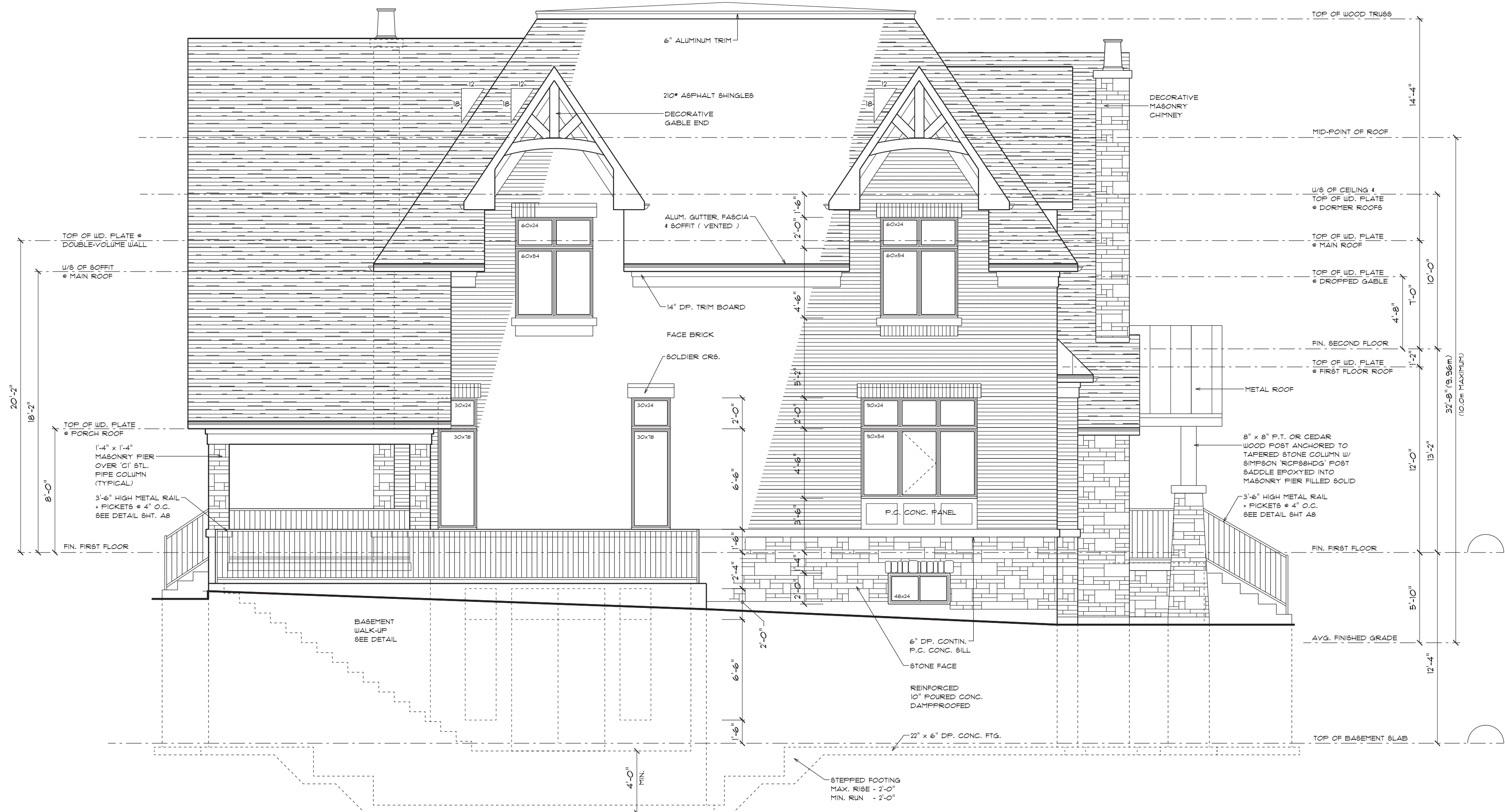
LEFT-SIDE ELEVATION BUILDING FACE AREA - 1084.2 SQ. FT. UNPROTECTED OPENING AREA - 138.8 SQ. FT. (12.8%) NOTE - LIMITING DISTANCE CALCULATED USING GLASS AREA ONLY.
