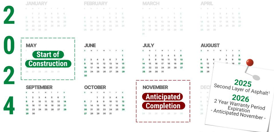
1. The second layer of asphalt is typically placed a year after the first layer, in case there are any defects in the first layer of asphalt, such as settlement. This allows us time to identify any defects and correct them before the second layer (top course) of asphalt is placed.
